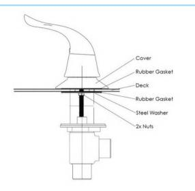
1. Unscrew the 2 nuts securing the steel washer and rubber gasket. In this order, remove the steel washer and rubber gasket, place your lever on the deck, replace the rubber gasket and the steel washer. Firmly secure the 2 nuts to hold the fixture in place.
