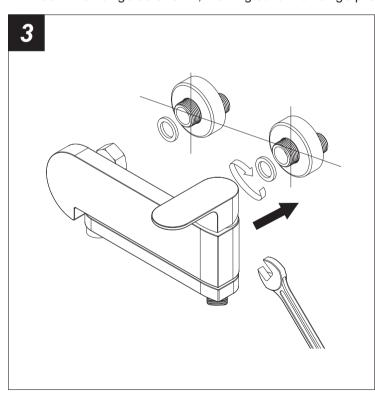
3.Install the faucet to the eccentric nuts as shown. Adjust the eccentric nuts if they do not match properly. Finally tighten by wrench.
