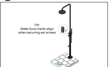
Insert top shower pipe (1) into bottom shower pipe (2). Connect hex head end of hose to swivel joint and tapered end to handshower (4). Place the tapered end of the hose into the handshower holder (9).
