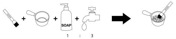
Open the gas cylinder valve. Small bubbles will appear where there are leaks.
