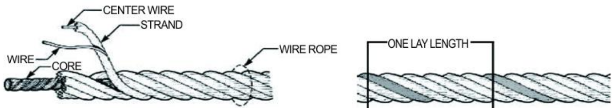
The three basic components of a typical wire rope.
