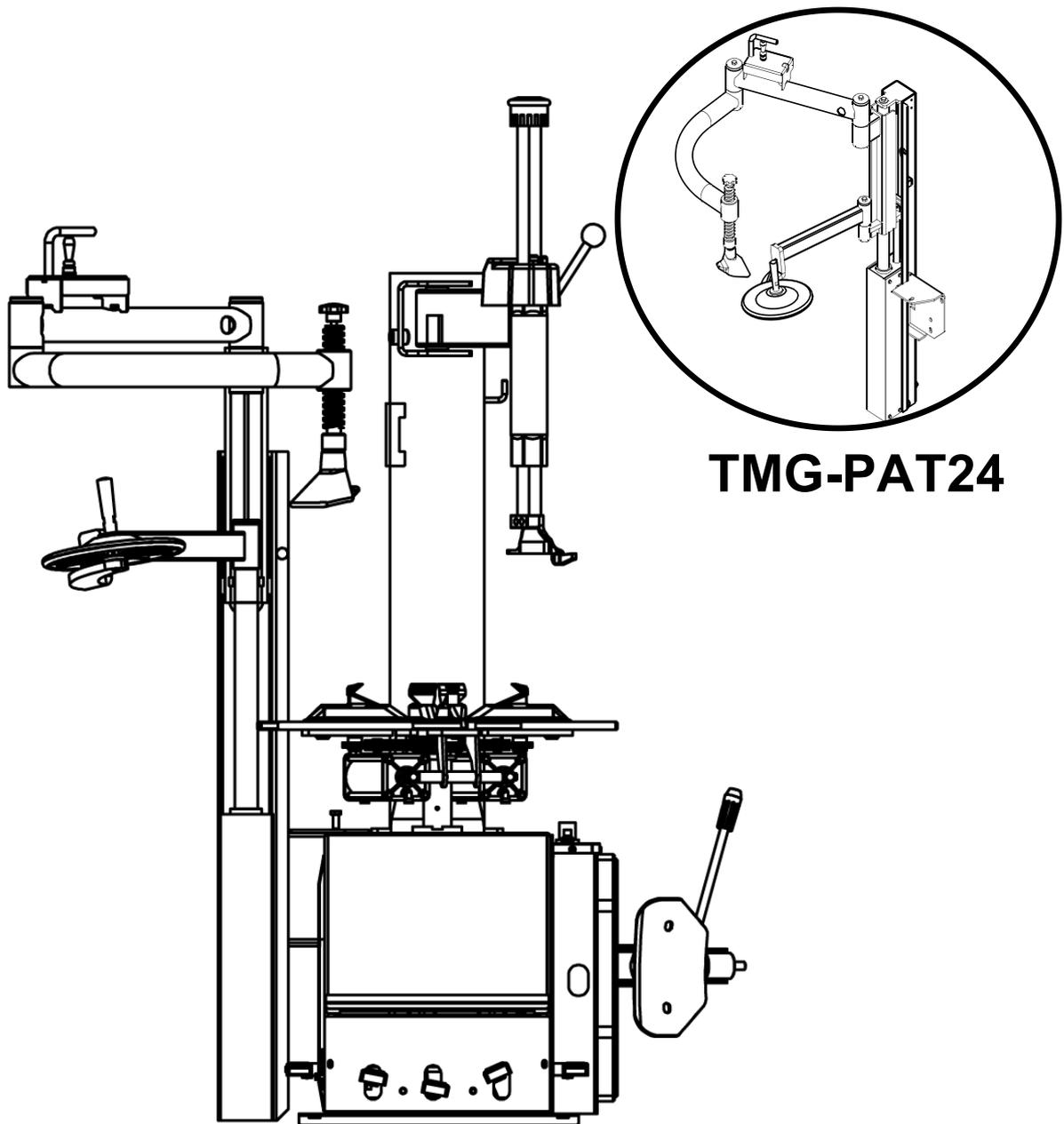
Pneumatic Assist Arm (**TMG-PAT24**) include TIRE-PRESSING BLOCK, TIRE-LIFTING DISC, it can easily dismount Run-flat and Low-profile tires, practical and saving space
