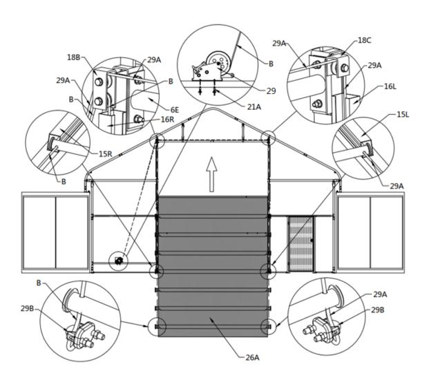
Now the door can be opened or closed by operating the winch assembly. Run the door up and down a few times to make sure all dropping tubes are moving smooth. Use lubricant oil if needed.
