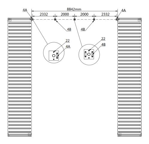
Installation diagram of expansion bolt.
