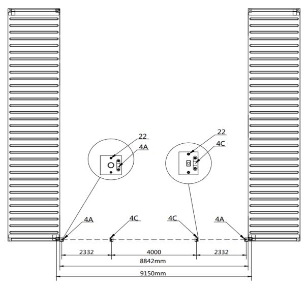
Installation diagram of expansion bolt.
