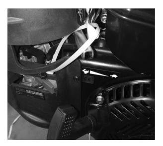
3) Retractable start: Slowly pull starter handle until just past compression-STOP! Return starter handle, firmly pull straight out to avoid excessive rope wear from starter guide.
