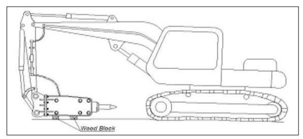
2) Turn the shut off valve (installed to the end of the boom arm) 90 degrees to the "off" position to prevent the hydraulic oil from flowing out.
