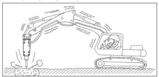
On the contrary, when position is excessive enough to break rocks with the front of the base machine raised, the machine may suddenly tilt forward the moment rocks are broken. Then, the breaker body or the end of bracket may violently hit against rocks and result in damage.
