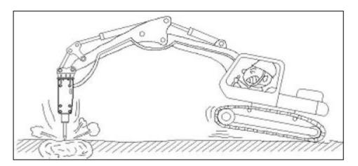
It is undesirable to carry out hammering under the below condition, because vibrations during hammering may be transmitted to the tracks of the base machine. During hammering, however, proper position must be always applied to the breaker. Special care must be taken not to hammer under abnormal condition.
