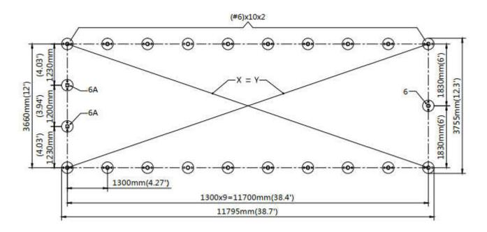
• Installation diagram of expansion bolt.
