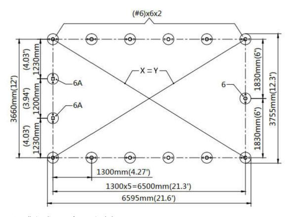
Installation diagram of expansion bolt.
