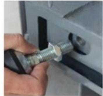
3. Place the platform scale at the desired location (room corners are recommended to prevent people from tripping). Adjust feet height with a flat screw driver to ensure the platform is leveled (see picture). Once the platform scale is leveled, tighten the nut on each foot glide.
