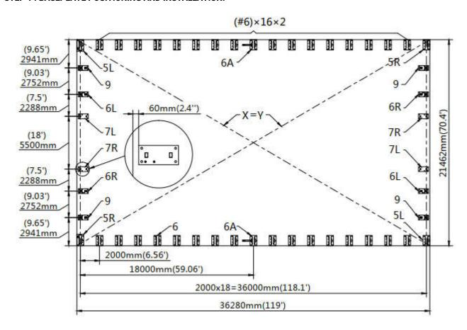
Installation diagram of expansion bolt.
