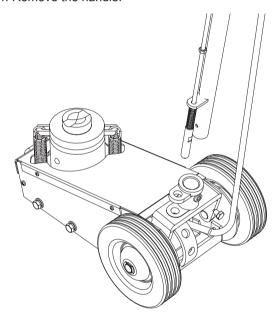
5. Turn the jack on its side so that old oil will drain from the oil fill hole.
