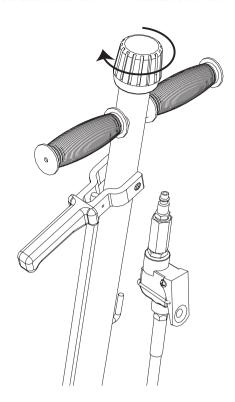
3. When the saddle reaches Max. Lift Height, then turn the handle knob counter-clockwise.
