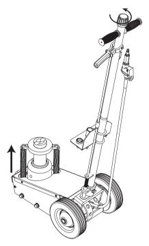
4. When the saddle reaches Min. Lift Height, with a flat blade screwdriver, push the oil fill plug slightly to the side to purge trapped air from system.
