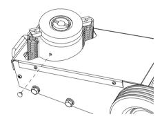
3. Fill the oil case until oil level is just beneath the lower rim of the oil fill hole.
