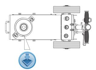
Fill the oil case until oil level is just beneath the lower rim.
