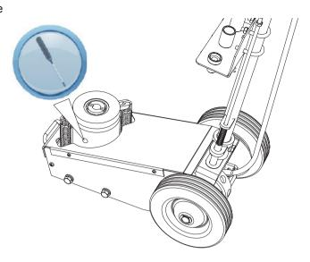
5. Close the release valve by turning the handle knob clockwise until firm resistance is felt.
