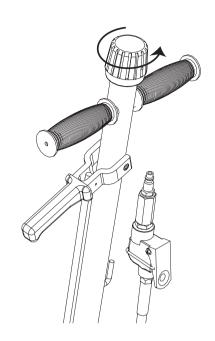
5. After removing jack from under the load, push ram and handle sleeve down to reduce exposure to rust and contamination.
