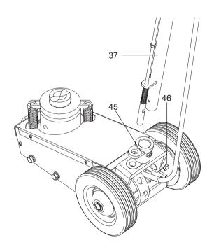
Carefully place the adapter plate (40) onto the handle (37) with U-bolts (44), washer (43), lock washer (42) and nut (41). Place extension adapters on the plate and secure with spring clips (39).
