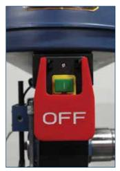
SAFETY LINE INTERRUPT switch requires manual reset in case of power loss.
