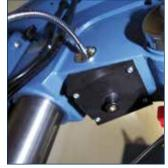
BUILT-IN LASER PROVIDES precise repeat drilling at any angle.
