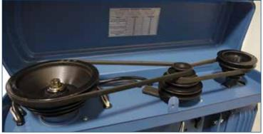
CAST IRON PULLEYS reduce vibration. Speed changes are quick and easy.
