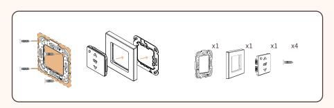
Begin installation of wall switch by installing the mounting bracket with each of the 4 provided countersunk screws. (Installing wall switch near a metal frame will impact performance of remote.)
