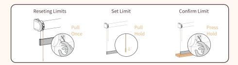
**Reseting Limits:** Reset limits by pressing the program button on shade motor. The shade will jog up and down, continue to hold until shade jogs up and down for a second time. New limits are now ready to be set.
