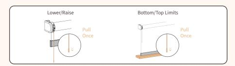
**Lower/Raise:** Lower shade by pulling once on wand to lower an again to stop. To raise shade pull once on wand and to stop pull once more.
