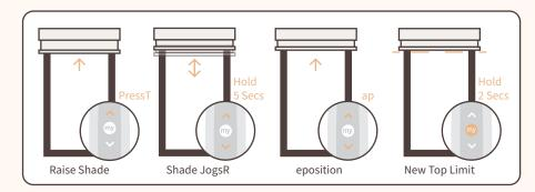
**Setting Top Limit:** To adjust the top limit, raise the shade to the preset top position. Press and hold the up and down button simultaneously until the shade jogs. Reposition the shade to the desired top limit. Press and hold the My button for 2 secs to confirm the new bottom position. The shade will then jog, confirming position.
