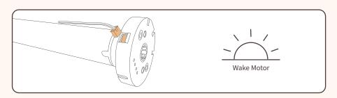
Activating Motor: When shipping the shade will be placed in a sleep mode. Wake up shade by connecting the motor to the charger. The shade will briefly jog up/down. Motor will now operate with programed transmitter.
