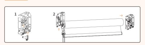
**Step 1:** Before installing shades, bearing pins must be installed in to bracket.
