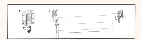
**Step 1-2:** Before installing shade, install bearing pins to the brackets. To install shade slide bearing pin side of shade in first. Then begin to slide the chain side up in to bracket.
