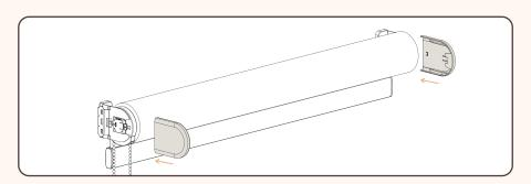
Once successfully installed place the bracket coverings on the roller shade brackets.
