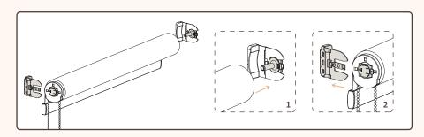
Begin with installing bearing pin side first, once fully inserted slide in the control side until you hear a slight click.
