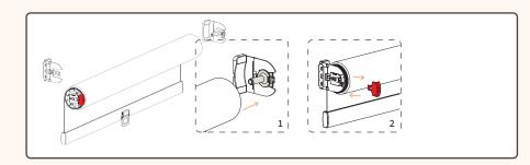
Begin with installing bearing pin side first, once fully inserted slide in the side with red clip. The red clip will pop off the shade once the shade is installed. Please note the red clip should not be taken off prior to installing on to bracket.
