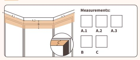
**Step A:** Measure the desired width from the left side of the window opening to the start of the first break in your bay window. Then measure the inside breaks. Then Measure from inside break to right desired width.
