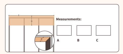
**Step A:** Measure the width from wall to wall. Subtract 1" from total for toarence.
