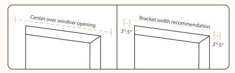
**Finding the Width:** Begin by taking the width measurement of your Cornice and center it over the window opening.
