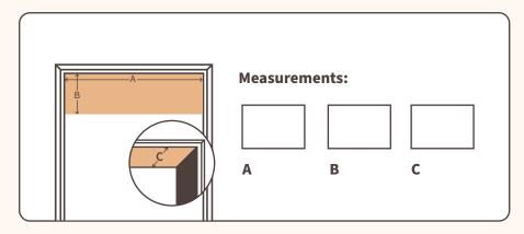
**Step A:** Measure the top inside width of window opening.
