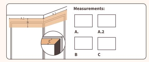
**Step A:** Measure the desired width from one end of opening to the corner. Then do the same to the other half of opening.
