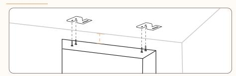
**Ceiling/Jamb Reduced Cap:** Typically mount directly to the ceiling or inside the window jamb.
