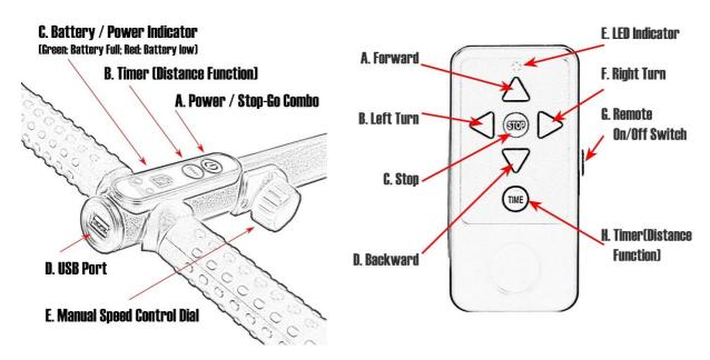
**Power ON/Off.** Press and Hold handle's A. Power/Stop-Go Combo button for 3-5 seconds to turn the cart power ON or OFF. During the manual control mode, briefly press the POWER button to Pause or Replay the cart.
