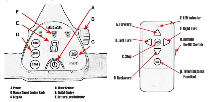
**Power ON/Off** Press and Hold handle's A. Power button for 3-5 seconds to turn the cart power ON or OFF. The battery LED will illuminate, when Power is ON.
