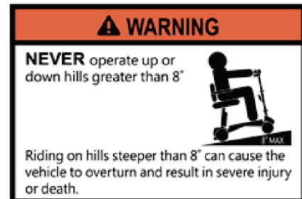
Maximum Incline Warning Label
