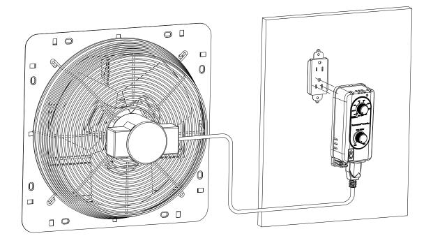
3. Hardwire a power cord to the fan. Plug the power cord of fan into the socket of Thermospeed control to get power.
