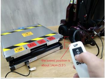
7. Note: we have included 2 elastic band for you to secure the scooter when it is placed on the platform during upraising and down ward operation of the lift. It is a good practice to always secure the scooter when it is on the platform.
