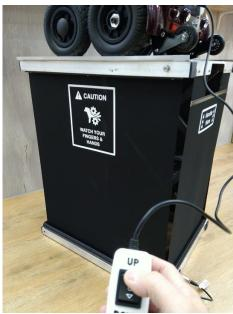
6. Press the down arrow to lower the lift.
