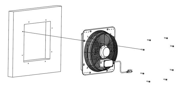
3. Please ensure the space has a gap for enough air to get into the space. The fan installed on free space of at least 4 inches above the upper edges of the corner.
