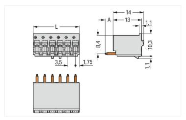
Dimensiones en mm L = pole no. x pin spacing A = 3.6 mm THT solder pin A = 2.4 mm THR solder pin
