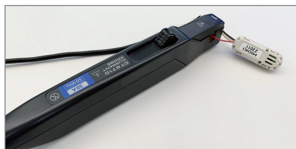
Fig. 26. Example measurement of the current consumption of a temperature and humidity sensor.
