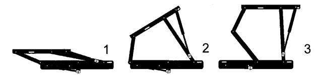
With this set of hinges you can use as traditional storage bed since the anchor and opening of the mechanism is identical to the standard hinged.
