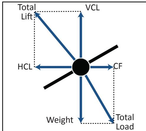
In a slipping turn, the HCL is greater than the CF. This is because the rate of turn is too slow for the angle of bank. The aircraft is yawed to the outside of the turning flight path in a slipping turn.
