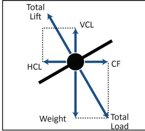
Because weight is unchanged in a bank and vertical lift (VL) is decreased (since some VL becomes HL) the aircraft will lose altitude; weight now exceeds the VCL (Center Graphic).
