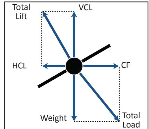
In a skidding turn, the CF is greater than the HCL. This is because the rate of turn is too great for the angle of bank. The aircraft is yawed to the inside of the turning flight path in a skidding turn.
