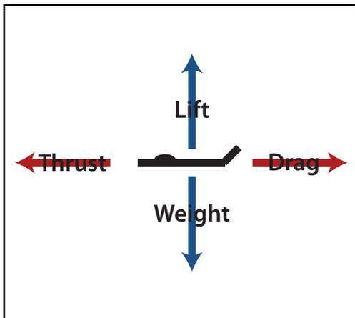
In straight and level flight, lift is equal to weight and thrust is equal to drag. Airspeed and altitude do not change.
