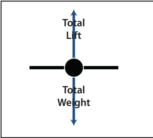
As shown above, in straight and level flight, Lift is equal to Weight. When banked, total lift banks with an aircraft while Weight continues to point toward the center of the Earth (Center/Right Graphics).
