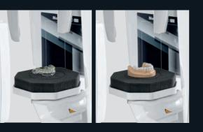
A specific protocol allows for tomographic scans of radiological templates, prostheses, models or impressions after they have been positioned on a special support.
