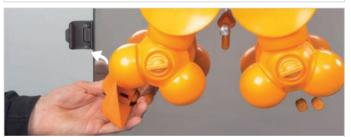
5. Pull off the peel ejectors.
