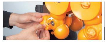
**13.** Fix the knobs and tighten them well. Missing knobs are to be replaced immediately. Never operate the machine with any knob missing.
