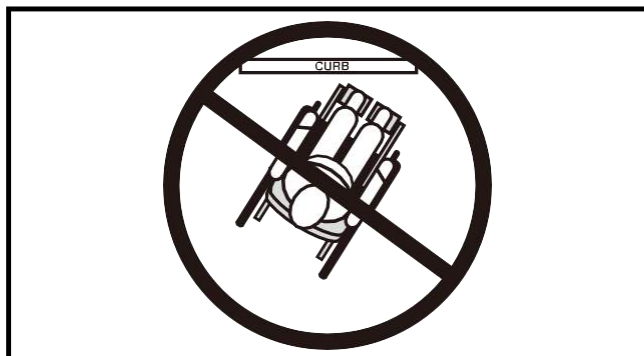
Figure 3. Incorrect Curb Approach
