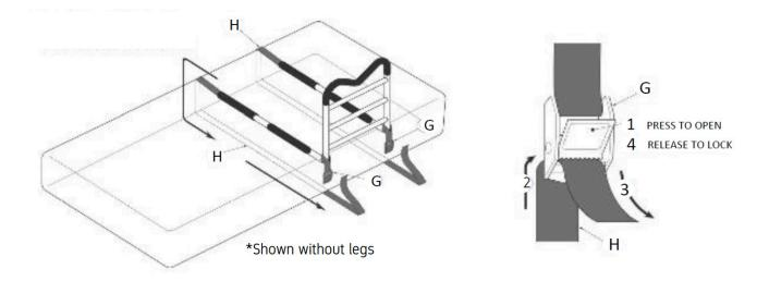
IMPORTANT: For your safety, the part H safety strap set provided with this bedrail MUST be installed as shown above.
