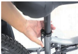
Adjust the height and direction and lock the buckle
