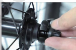
Both sides must be tightened, pull up the safety lock
