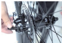
Tighten the thru-axle screw
