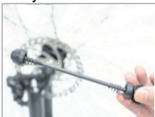
Install the front wheel into the fork
