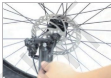
Pass the thru-axle through the front fork and front wheel
