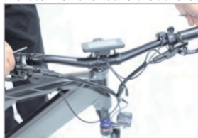
Put the handlebar on the stem
