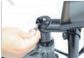
Next fix the two screws on the side of the stem
