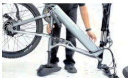
Release the thru-axle screw
