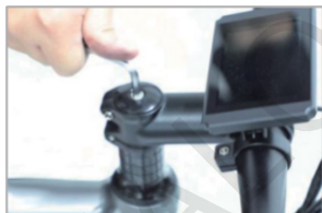
First fix the upper middle screw of the stem
