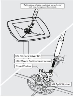
Locate and secure the Case onto the Mounting Arm as shown. Tighten by
