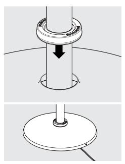
With the Floorstanding Cover on the ground, locate and fit the Floorstanding Rubber Collar.
