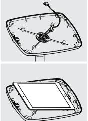
7 Install the tablet into the Case & connect to power.
