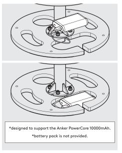
9.2 If installing a battery pack, connect the tablet cable and locate the pack into the Floorstanding Base.
