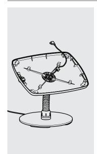
Feed the tablet cable through the Bouncepad Case & mounting arm
