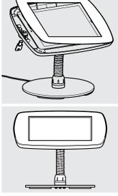
6 Locate and lock the Faceplate onto the Bouncepad Case.
