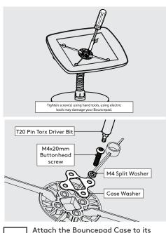
Attach the Bouncepad Case to its Mounting Arm. Take care to ensure correct & full thread engagement.
