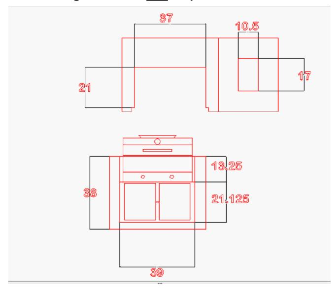
Above drawing shows a 38" tall counter with a 2" thick top. 10.5"x17" dimensions on top image show the cutout required for optional sideburner.
