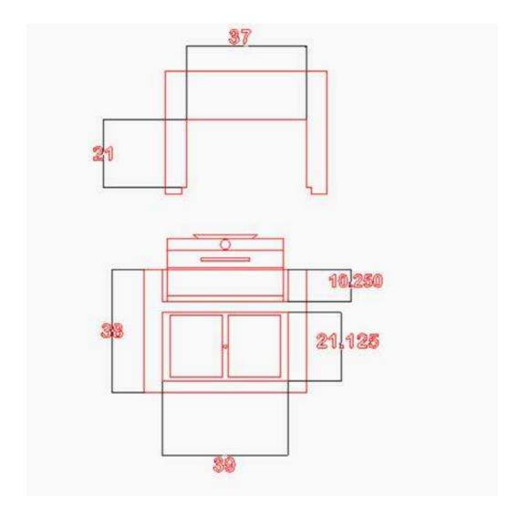
Above drawing shows a 38" tall counter with a 2" thick top. 10.5"x17" dimensions on top image show the cutout required for optional sideburner. An open grill lid will require a 12" clearance beind the grill on the counter.
