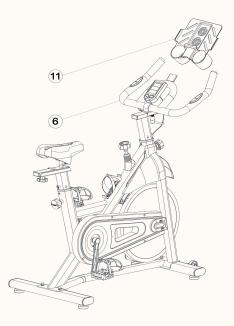
7. Install the tablet holder(11) on the Handle Frame (6) by sliding it in.
