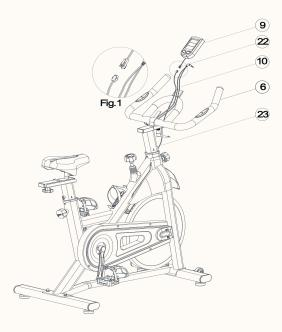
**6.** Insert the monitor (9) onto his mount in the middle of the handle. Match the sensor wire A (22) and the sensor wire B (23).
