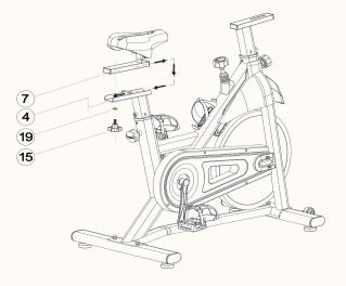
**4.** Slide the seat adjustment (7) on the seat post (4). Then secure it with a flat washer (19) and an adjustment knob (15).
