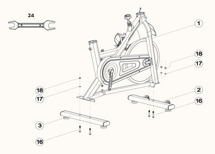
**1.** Fix the Front Stabilizer(2) to the main frame(1) with Carriage Bolts(16), Flat washers(17) and cover nuts(18). Tighten with open wrench(25).
