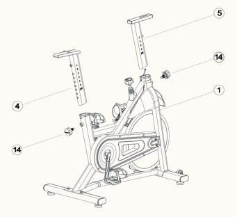
**3.** Insert the seat post (4) in the main frame (1) and screw the adjustment knob (14) to secure it. Repeat the same process with the handle post (5).
