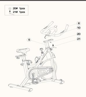
**5.** Put a washer (20) and then pass the threaded end of the L-shaped adjustment knob (21) through the adjustment slot of the handle post(5). Then place the handle (6) on top of the handle post and secure it by turning clockwise.
