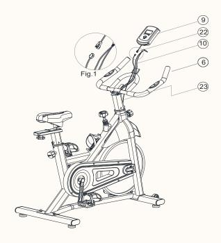
**6.** Insert the monitor (9) onto his mount in the middle of the handle. Match the sensor wire A (22) and the sensor wire B (23).
