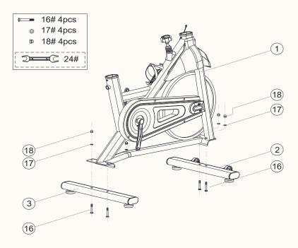
1. Fix the Front Stabilizer(2) to the main frame(1) with Carriage Bolts(16), Flat washers(17) and cover nuts(18). Tighten with open wrench(25).
