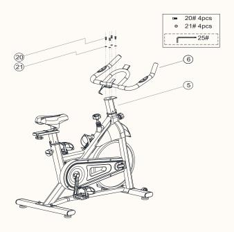
**5.** Fix the handle (6) on the handle post (5) with the spring washer (21) and the round head bolt (20). Tighten with the Allen wrench (25).
