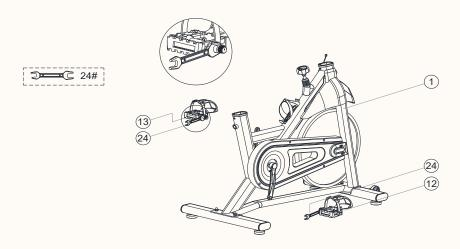
2. IMPORTANT INSCRUCTOIN! WARNING! When installing the pedals DO NOT use the wrench until you've done 4 FULL TURNS with your hand. If the pedals are not well installed this will damage the crank arm. (The Right and left sides are defined as if you were sitting on the bike)
