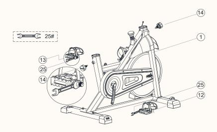
**3.** Insert the seat post (4) in the main frame (1) and screw the adjustment knob (14) to secure it. Repeat the same process with the handle post (5).
