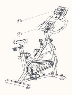
7. Install the Mobile phone holder (11) on the Handle Frame (6) by sliding it in.
