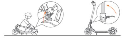
• Unfold the handlebar stem and close the quick-release lever.
