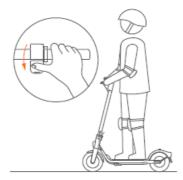
• Slow down by releasing the throttle and squeezing the brake lever. The rear light flashes when braking (not for F20D, F30D or F40D).
