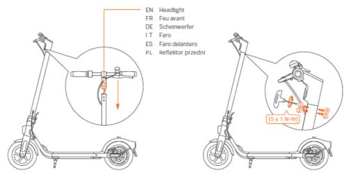
• Install the 4 screws in order (two on each side) with the included hex wrench.
