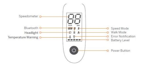
**Power Button:** Press the button to turn on; press and hold the button for 3 seconds to turn off. When the KickScooter is on, press the button to turn on/off the headlight and the rear light, and press twice to switch between the speed modes.
