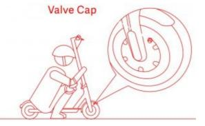
2. Connect the extension nozzle to the tire valve stem.
