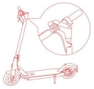
3. Tighten the screws onto both sides of the stem with the T-shaped Allen key.
