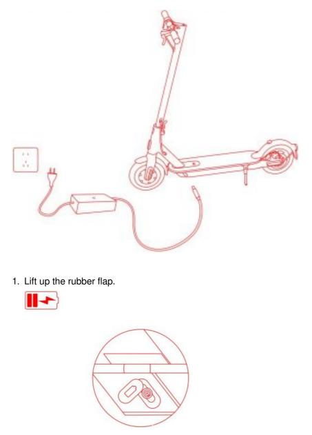
2. Plug the power adapter into the charging port.
