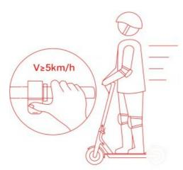
4. Release the accelerator and squeeze the brake lever for a sudden brake.
