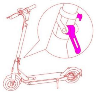
2. Install the handlebar onto the stem.
