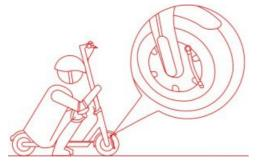
3. Connect the pump to inflate the tire.
