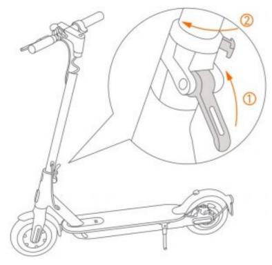
2. Install the handlebar onto the stem.
