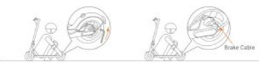
Before adjustment, make sure the scooter is powered off and not charging. If the brake is too tight/loose, use the 4 mm Allen key to loosen the screw on the caliper. Then slightly adjust the brake line (decrease/increase the exposed lenght), and tighten the screw again.
