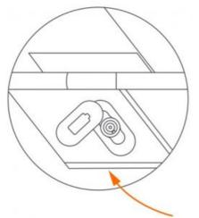
2. EN Plug the power adapter into the charging port.
