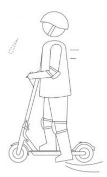
4. The accelerator initiates once the coasting speed exceeds 5 km/h.
