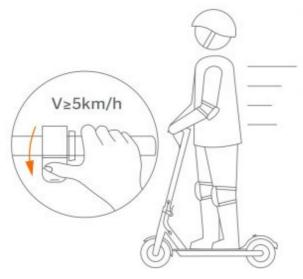
5. Release the accelerator and squeeze the brake lever for a sudden brake.
