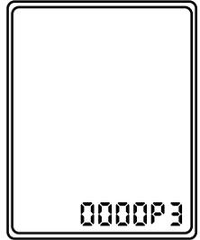
**Attention** If the user changes the power-on password, please be careful to remember it; if you forget your password, Press and hold the M button and the “-” button for 2 seconds to reset the factory password.
