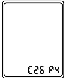
button into P4, press the “+/-” buttons to change the wheel diameter.
