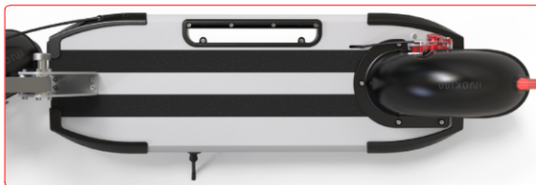
ALUMINIUM DECK WITH CARRY HANDLE + ANTI SKID GRIPS
