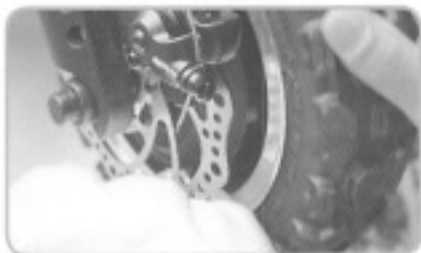
[4] Wipe the inner side of the disc while rotating the wheel.
