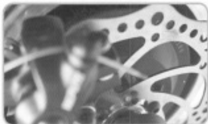
[2] There is a stripe on the part where the pad touches, but it does not look dirty when you see it with your eyes.
