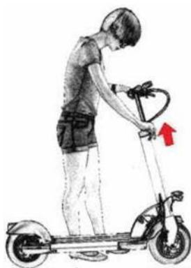
Rotate the handlebar lock lever and raise the bar to the desired position. Once raised, squeeze the lever.
