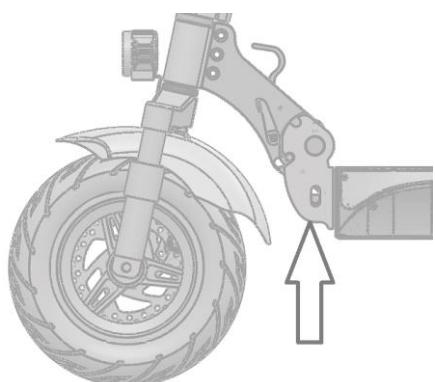
In case you feel vibration in the handlebar/stem, please use the hex key to adjust the folding/unfolding mechanism of the scooter.
