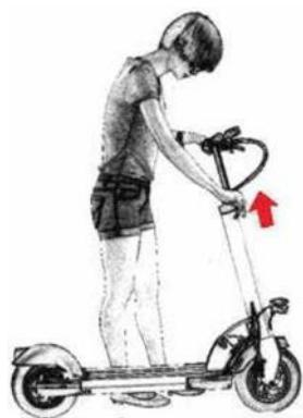
Rotate the handlebar lock lever and raise the bar to the desired position. Once raised, squeeze the lever.
