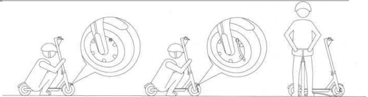
Make sure the tires are properly inflated. These can be inflated with a bicycle pump. Once inflated, be sure to put the valve caps on.
