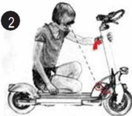
Raise the lever to lock the fold handle while firmly holding the fold bar.
