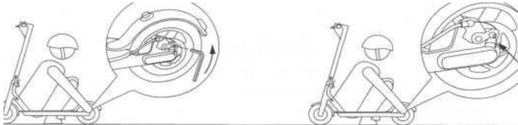
If the brake is too tight or has play, use an M5 hex wrench to adjust accordingly and push the pistons back in as far as possible, being careful not to bend them. Do not push the pistons with a sharp tool, as this may damage them and cause further damage.
