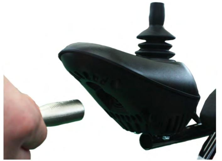
Charging directly to the wheelchair while battery is connected to the wheelchair (sold seperatly)
