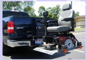
US208P has a pocket for Mid- Drive Mobility devices to rest in for secure travels.
