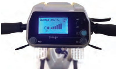
Multi-feature digital dash/LCD display with easy read user controls
